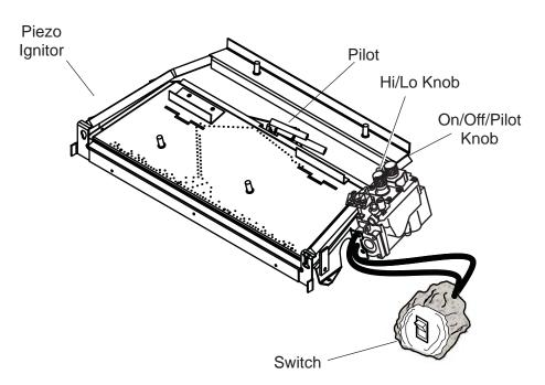
Figure 33 - Location of Piezo Ignitor, Control Knobs and Switch
